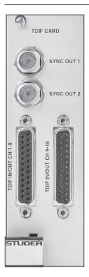
This card provides two eight-channel TDIF I/O interfaces with 96 kHz, 88.2 kHz, 48 kHz, or 44.1 kHz operation with wordclock sync outputs on BNC connectors. Inputs and outputs are provided on standard 25-pin D-type connectors (female).
