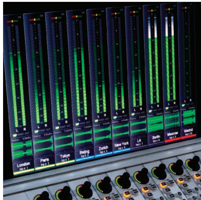
Comprehensive metering on the Vista X control surface.
