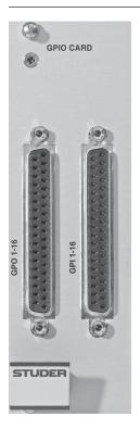
For general-purpose applications requiring total electrical isolation, this card provides 16 electrically isolated opto-coupler inputs with integrated current sink (5-24 VDC) and 16 electrically isolated outputs using SPST relay contacts. 5 VDC supply pins are available. Inputs and outputs on standard 37-pin D-type connectors (female).
