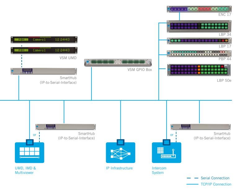
VSM servers are the heart of the control system. Running vsmStudio software, all administration and configuration is both programmed and saved runtime in intuitive and easy to use software. Control interfaces in the form of a wide range of hardware LCD button panels and software panel clients allow simplified operation from highly flexible and custom designed configurable GUIs.
