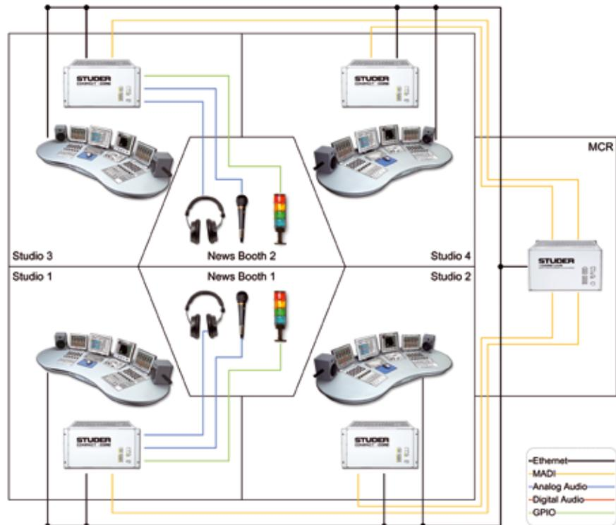
signal from Booth 2, while Booth 1 is at the same time used for the news with Studio 1. The setup also allows a very flexible emergency switch-over, since every studio can connect to any voice booth.
